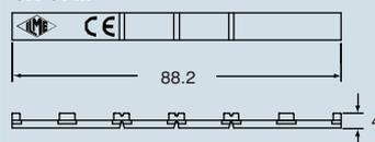
the modular units inserts must be installed in suitable frames which in turn are installed in traditional housings or COB panel support. Alternatively, individual modules with a width of 14.7, can be installed in plastic supports.
