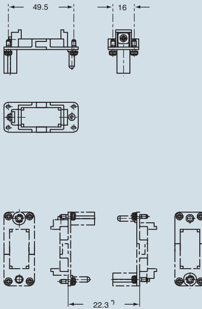
\*) distance for electric contacts: max 24 mm
