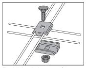
For joining in bottom of tray: 2 pcs of Fitting B2 1 pc of Bolt and Nut B13.
