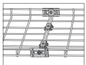
Wire tray 422 is joined with 2 pcs of Fitting B1 6 pcs of Fitting B2 4 pcs of Bolt and Nut B13
