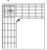
Wire tray 53 to 220 are joined with: 2 pcs of Fitting B1 2 pcs of Fitting B2 2 pcs of Bolt and Nut B13
