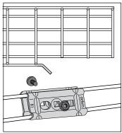
To obtain a softer inner angle, 2 Fittings B1 can be mounted with Bolt and Nut B13.
