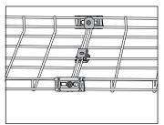
Wire tray 320 is joined with 2 pcs of Fitting B1 4 pcs of Fitting B2 3 pcs of Bolt and Nut B13
