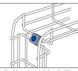
Vertical bends are joined with one or more Fitting B3, depending on wire tray width.
