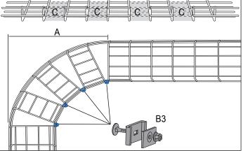
Wire tray 120-622 is shaped to straight 90 ° angle by cutting out every other marked wire tray section and joined with Fitting B3 according to table below.
