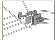
Horizontal bends are joined with Fitting B3.
