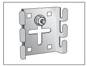
Mounted to wall/ceiling/floor with Expansion bolt in middle hole or screws in corner holes.
