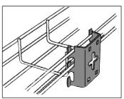
The side wires of the tray are easily hooked onto the grips of the bracket.
