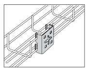
For horizontal mounting with bottom or side of tray onto the bracket grips.
