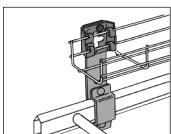
Wire trays are mounted onto Combi Fitting B21 with Bracket B4 or B4 Mini.
