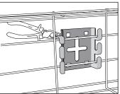
For increased stability, the B4 grips can be closed around the wires.
