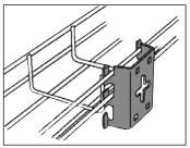
The side wires of the tray are easily hooked onto the grips of the bracket.
