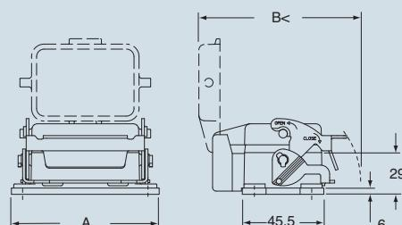
**NB:** the enclosures ensure IP66 protection (or IP65 cover versions) rating when mated and locked with the closing levers.
