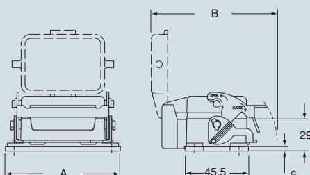
**NB:** the enclosures ensure IP66 protection (or IP65 cover versions) rating when mated and locked with the closing levers.
