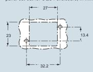
panel cut-out for CQS IA - CQS IAP enclosure, in mm
