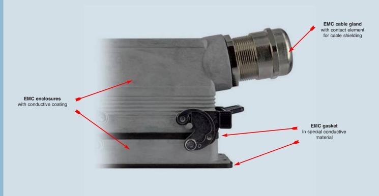
The enclosure surfaces are treated to make them extremely conductive while maintaining the necessary corrosion resistance.
