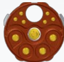
11-polig Stift E Code 1 11-pin male contact E Code 1 (5 X Ø 2 mm (4 + PE) + 6 x Ø 1 mm)
