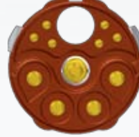
11-polig Stift E Code 1 11-pin male contact E Code 1 (5 X Ø 2 mm (4 + PE) + 6 x Ø 1 mm)
